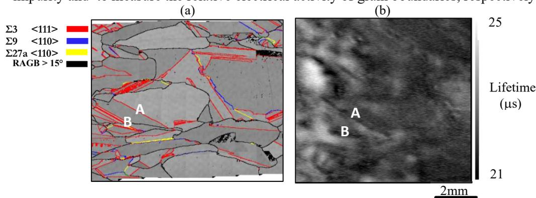
**Figure 1:** Silicon sample grown by cold crucible casting process : (a) CSL map showing different grain boundary types; (b) lifetime map obtained by microwave phase shift, without surface passivation. The scale is the same for (a) and (b). A: active  $\Sigma 3$  twin grain boundary, B: active random angle grain boundary.
