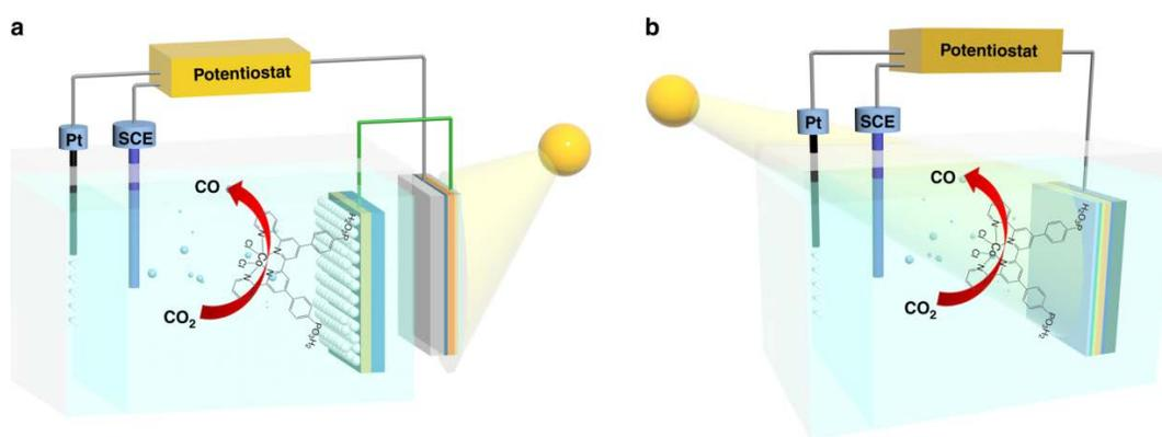
**Figure 1 Photo-assisted cell systems.** PV-EC system (a) and PEC system (b).
