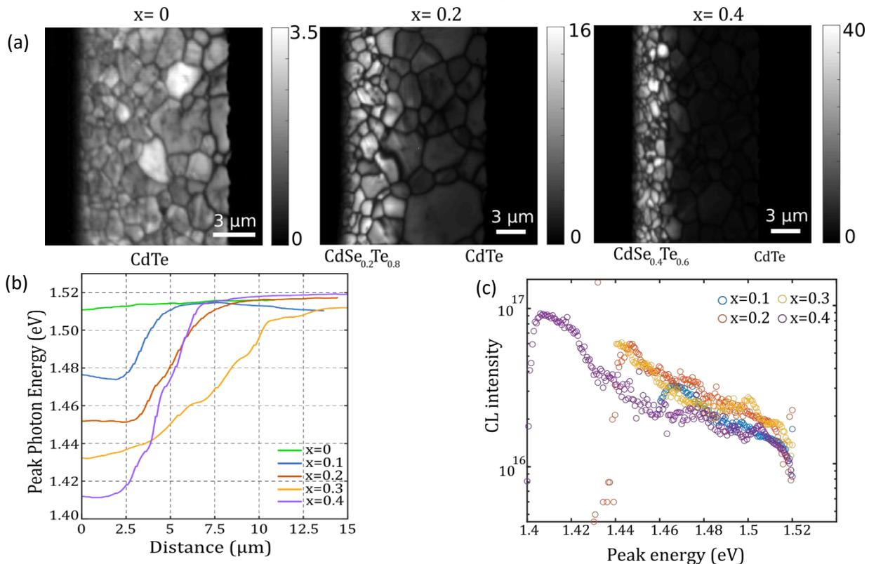
Figure 1 : CL intensity of CdSeTe sample with Se concentration ranging from 0 to 40%. (b) Peak photon energy as a function of distance from the CdSeTe/back contact interface along the surface. (c) Radiative efficiency as a function of the peak energy (logscale)
