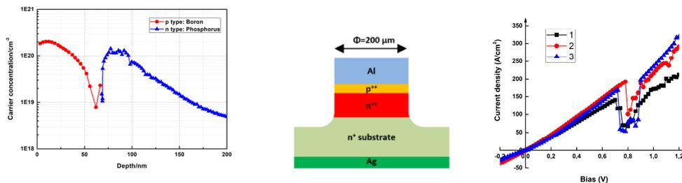
FIG.1. Carrier concentration of a  $p^{++}/n^{++}$  type tunnel junction measured by ECV. Schematic and I-V characteristics of  $p^{++}/n^{++}$  single tunnel diode on (111) Si substrate
