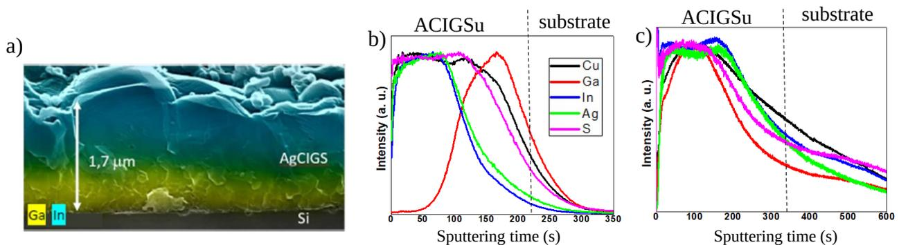
**Figure 1:** a) SEM cross section of Si/Ag-Cu-In-Ga sulfurized at 600°C, with EDX color mapping, b) GDOES analysis of ACIGSu sulfurized at 600°C, c) GDOES of ACIGSu sulfurized at 700°C, with normalized intensities.
