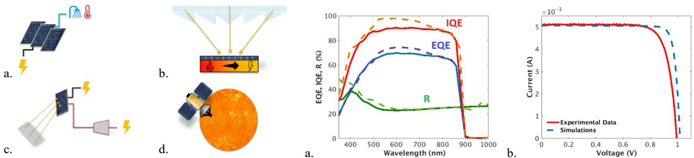
Figure 1. Solar cells operating under thermal stress in: (a) photovoltaic-thermal, (b) photovoltaic-thermoelectric, (c) photovoltaic-CSP terrestrial hybrid systems, and (d) near-the-sun space missions.
