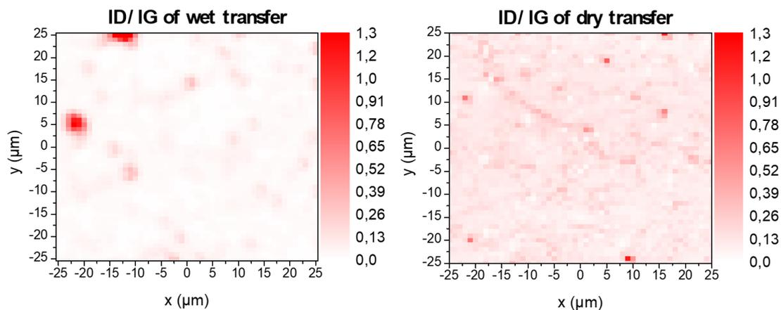
Figure 1 ID/IG Raman peaks ratio of graphene transferred by the wet and dry methods. The larger averaged ratio for the dry method indicates a low-quality graphene.
