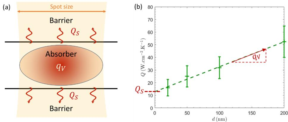
Figure 1: (a) Sketch illustrating the surface ( $Q_S$ ) and volume ( $q_V$ ) contributions to thermalization under illumination. (b) Thermalization coefficients measured as a function of the absorber thickness. The intercept corresponds to the surface contribution while the slope gives the volume contribution.
