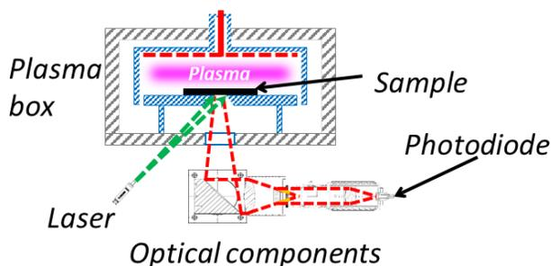
Figure 1: In-situ MPL setup with PECVD chamber
