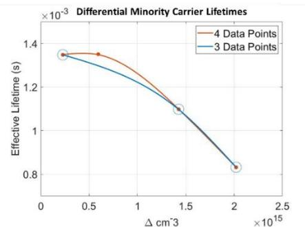
Figure 2: Effective carrier lifetime as a function of excess carrier density.
