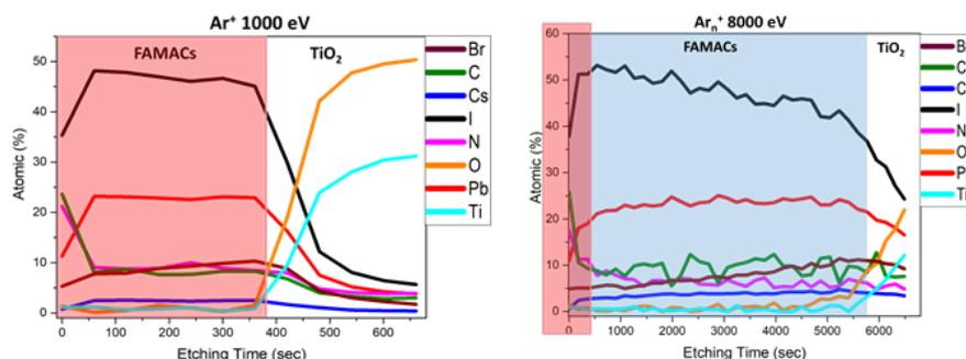
Figure 1. XPS depth profile of FAMACs perovskite layer deposited on FTO / TiO<sub>2</sub> substrate using Ar<sup>+</sup> (left) and Ar<sub>n</sub><sup>+</sup> (right) ion sources
