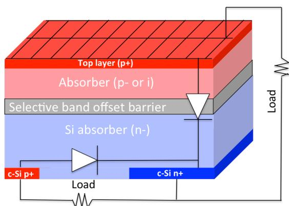
**Figure 1** Three terminal band offset barrier tandem solar layer (3T-SBOB). The absorber in this work is perovskite.
