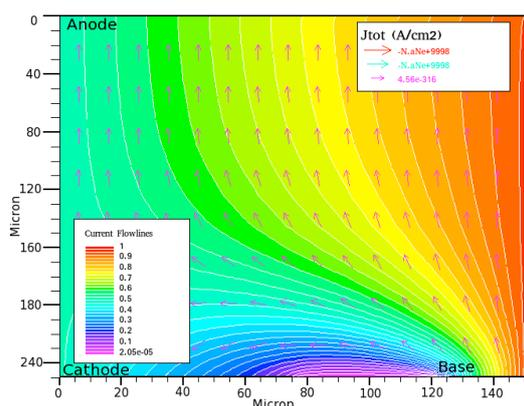
**Figure 3** Current flow lines over the device for a thick IBC. The PSC is not resolved at this scale.
