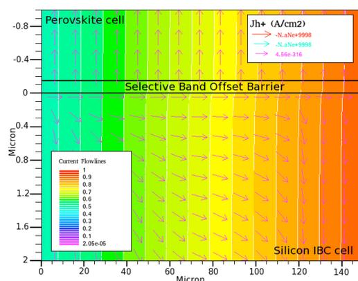
**Figure 4** A zoom showing only the hole current flowlines over the top section of the 3T-SBOB. The IBC holes are seen to be repelled by the SBOB. Holes in the top cell are collected at the front contact.
