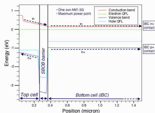
**Figure 2** Numerical simulation of the band structure of the spectrum 3T-SBOB device under one sun illumination. The band offset in the valence band prevents hole transport. Independent quasi-Fermi level separations form in the top and bottom cells.
