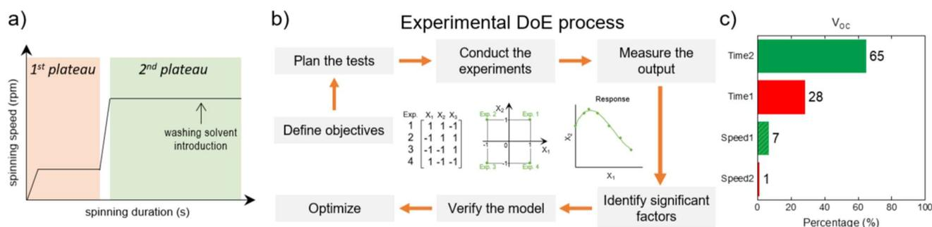
Figure 1: a) Scheme of the spinning speed evolution versus time for a 2-plateau 1-step spin-coating deposition b) Conceptual diagram of a DoE c) Example of the Pareto effect for the  $V_{oc}$ , where the colors are indicators of negative/positive impact of the parameters and the length, its the weight.
