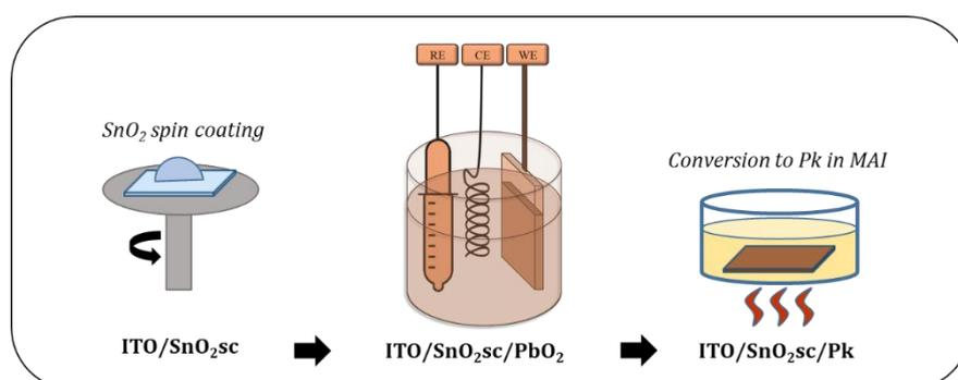
Figure 1: Steps followed to elaborate the perovskite layer presented in this work
