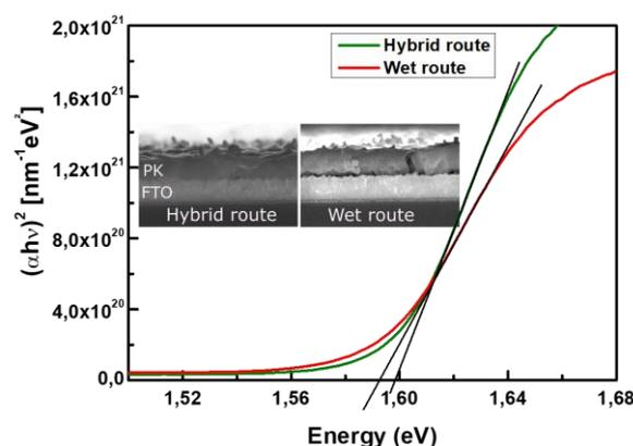
**Figure 1:** Tauc plots of PK deposited via Hybrid and Full-wet route on FTO glass yield quite similar bandgaps. Inset the SEM images showing different morphologies of the two configurations.
