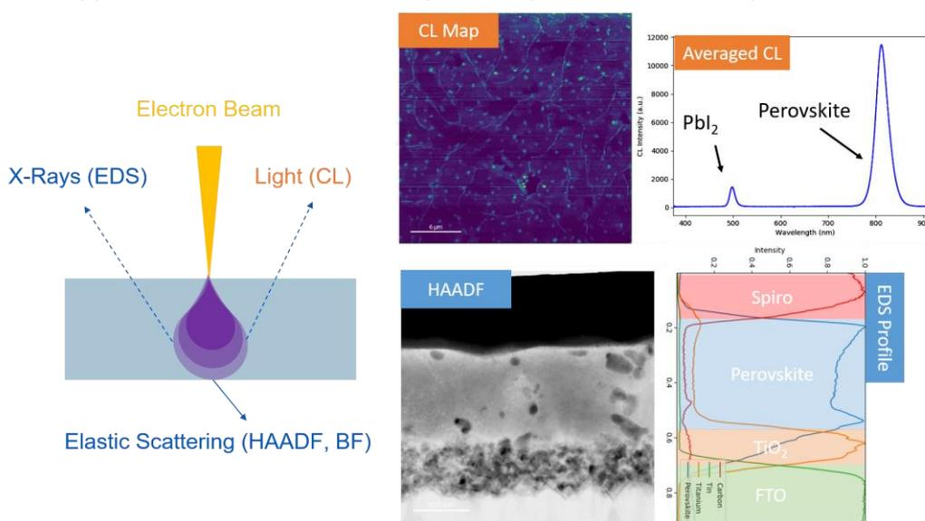
Figure – Representative Results using Electron Microscopy. A) Schematic of electron-material interactions. B) CL panchromatic map and CL spectrum averaged over the full area. C) HAADF image of perovskite cross-section and Element profile corresponding.
