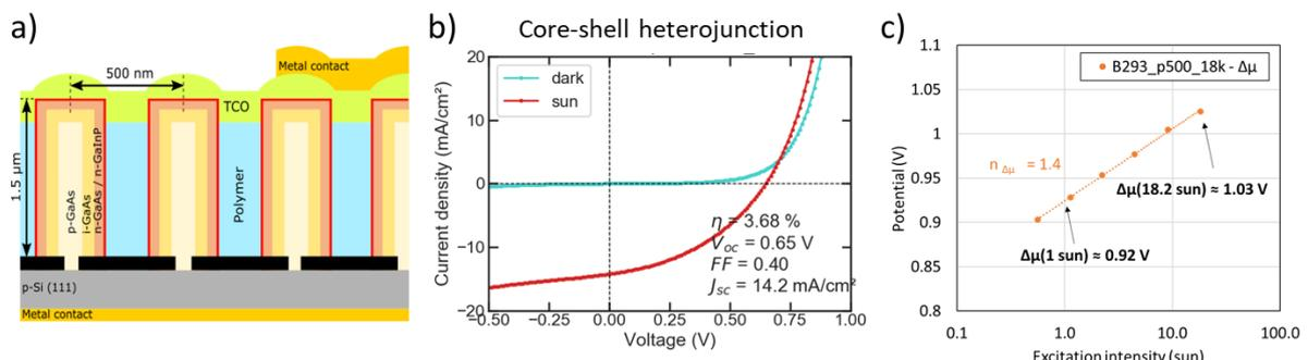
**Figure a)** Schematic of the NW-based top cell. **b)** JV-characteristics (dark and under AM1.5G) of a GaAs/InGaP NW core-shell heterojunction. **c)** Evolution of the quasi-Fermi level splitting (measured using a hyperspectral imager) of an as-grown heterojunction nanowire array with excitation intensity.
