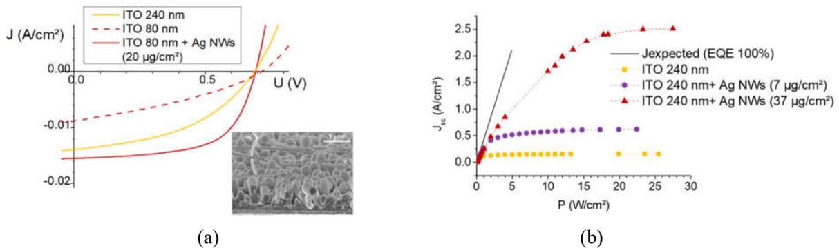
**Figure 1:** (a) JV curves under 1 Sun for a 7 mm<sup>2</sup> cell (inset: SEM cross-section with hybrid contact), (b)  $J_{sc}$  at different illuminating powers for Si/a-Si:H NW solar cells with and without Ag NWs.
