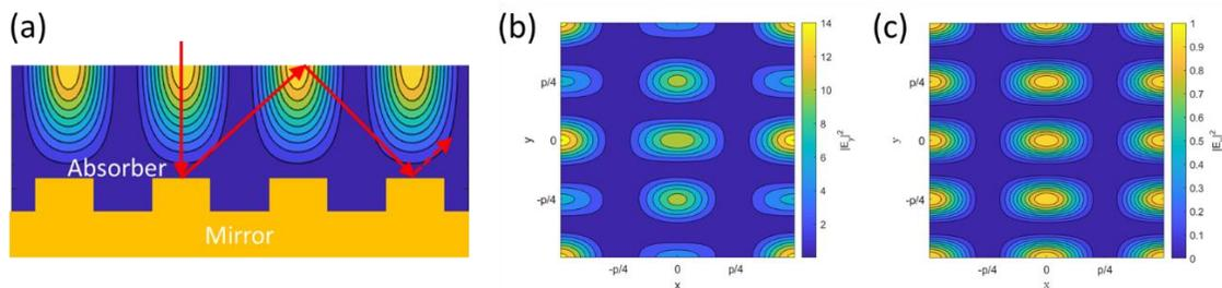
Figure 1: (a) We consider an ultrathin light absorber (100 nm) on top of a perfect mirror patterned with a 2D periodic grating. The grating can diffract incident light so that it can couple with resonant modes in the absorber. (b) Top view of the electric field intensity map obtained from a RCWA simulation at an absorption peak. (c) The same map as expected from our analytical model for the corresponding resonant mode. The shapes of (b) and (c) are in perfect agreement.
