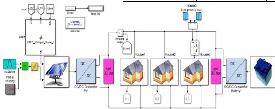
Fig. 1. Simulation model of a PV-based DC microgrid using components in Simscape Power Systems Toolbox.
