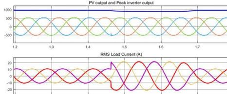
Fig. 2. Simulated PV array consisting fifty-six (56) PV panels and total output voltage of 812V: The small dip in PV output is due to the inverter's loading from 5kW to 10kW.
