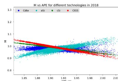
Figure 5 APE vs  $M$  values for CdTe, aSi, cSi, and CIS technologies with spectral measurements from 2018
