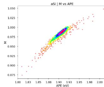
Figure 3  $M$  values corresponding to a-Si technology versus average photon energy and count of events.
