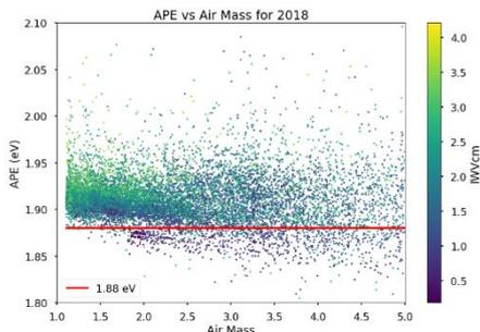
Figure 2 Average photon energy vs air mass and integrated water vapor on-site measurements for 2018
