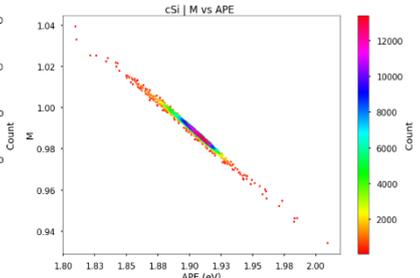
Figure 4  $M$  values corresponding to c-Si technology versus average photon energy and count of events.
