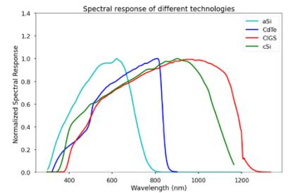
Figure 1 Spectral responses for different technologies normalized to their maximum value. Measured by CalLab PV Modules at Fraunhofer ISE.
