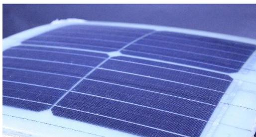
Figure 1 - Double-curved composite module produced by vacuum bagging process
