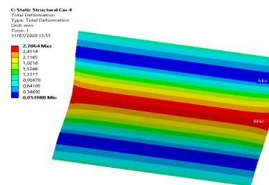
Figure 2 - Validation of the numerical model: simulation of the 3-point bending test
