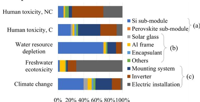
**Figure 1.** Contribution of each component of the perovskite/Si PV system to the ILCD categories in focus, i.e. climate change, freshwater ecotoxicity, water resource depletion and human toxicity, for 1 kWh of electricity produced by a perovskite/Si tandem module based slanted-roof installation. (a) Perovskite/Si tandem module, (b) PV panel (encapsulation, frame, module elements), where solar glass is also used as substrate of the perovskite sub-module, (c) BOS components.
