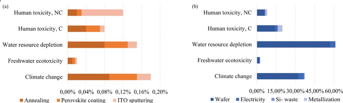
**Figure 2.** Detailed share of environmental impacts from the hotspots of (a) perovskite and (b) silicon sub-modules.
