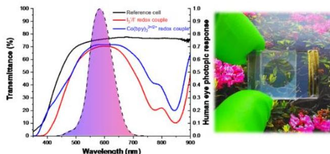
**Figure 1.** Transmittance spectra of full NIR-DSSCs based on VG20 dye (superimposed with the human's eye photopic response). On the right a picture of first proof-of-concept NIR-DSSC.
